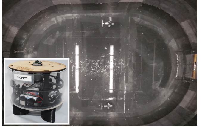
Fig. 1. An overhead view of the racetrack shaped experimental tank. The two propellers are visible at the top and bottom of the image, and a glass observation window is present on the right-hand side. Inset: a photo of the Modboat platform used for the experiments in this work. The Modboat is described in [6], and the controller used in this work is developed in [7].
